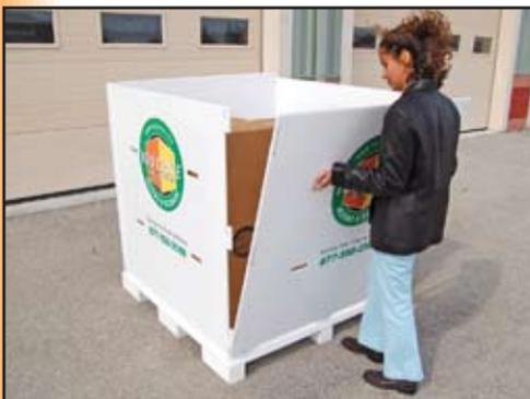
After loading the crate, insert the second side (C) into the matching slots of base (A). Fit side (C) slots over the extensions on (B) sides
