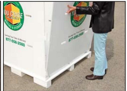
Insert the bottom of side (C) into the matching slots on the base (A). Fit side (C) slots over the extensions on (B) sides
